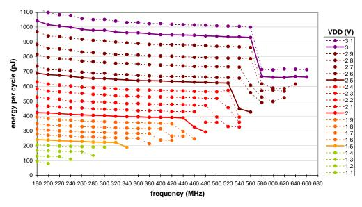
Figure 9: Energy versus frequency for various supply voltages. The results are typical energy per cycle as measured while executing the test program.
