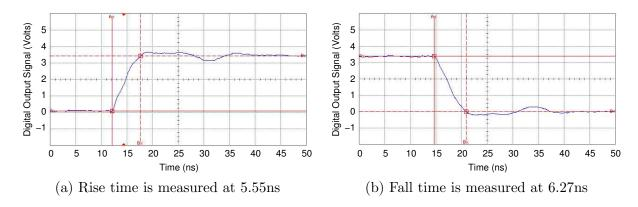
Figure 10: Full rail rise/fall time of STC1 digital output signal.
