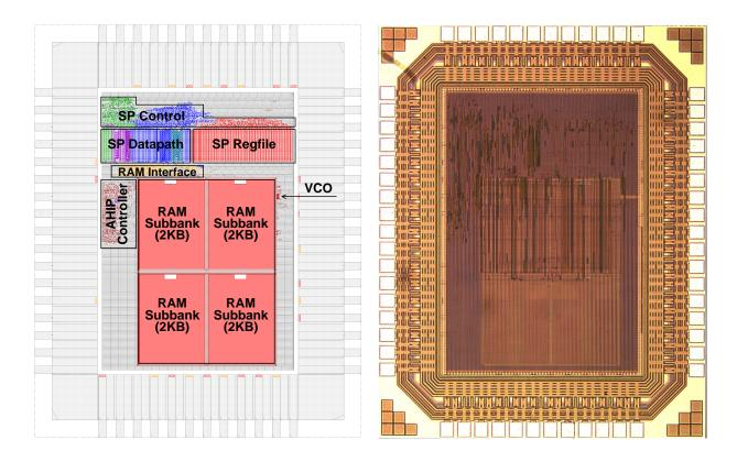
Figure 2: STC1 chip plot and die photo. On the chip plot, the Exec Unit is colored blue, and the Fetch Unit is colored green and purple.
