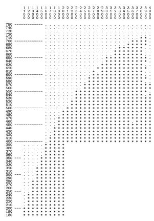
Figure 5: Shmoo plot for a wide voltage range. The horizontal axis plots supply voltage in mV, and the vertical axis plots frequency in MHz. A \* indicates correct operation at that operating point and a dot indicates failure. The shmoo plot shows combined results from two different chips.
