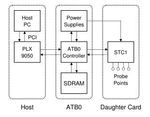
Figure 3: Test System Block Diagram. The test system includes the ATB0 test baseboard, a daughter card with the STC1 chip, and a host computer to control the test system.
