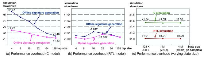
Figure 5. Performance evaluation of continual hashing in terms of simulation slowdown. We calculate and check the signature at every tick (i.e., for every sample) with 1 mega-sample frames. (a) shows the performance overhead caused by hash calculation and state inconsistency checking for reference C model and (b) for Bluespec RTL model. (c) shows that the performance overhead does not depend on the total state size as expected. For (c) tap\_size is 32 and the online scheme is used.
