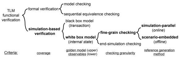
Figure 1. A taxonomy of TLM functional verification approaches. Our proposed approach is high-lighted in boldface.
