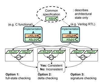
Figure 3. Three possible implementations of state consistency checking. At n-th checkpoint, each implementation dumps out the entire architectural state (AS[n]) for Option 1, the changes in the architectural state  $(\Delta AS[n])$  since the previous checkpoint for Option 2 and a signature (Sig[n]) for Option 3, respectively. The checker can detect a state inconsistency by comparing these dumped outputs.
