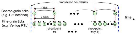
(c) State transitions of FIR module showing transactions, ticks and checkpoints
