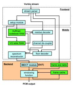
Figure 6. Functional modules of Vorbis decoder. Memory and computation modules are colored differently.
