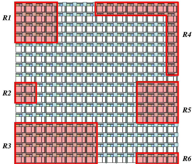
Figure 7-2: Illustration of using the operating system to allocate a collection of physical tiles for each independent program running on the CMP. The operating system is fully responsible for maintain cache coherence within different regions.
